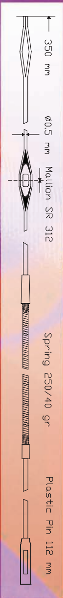
Stainless Steel Monowire Jacquard Heald with Spring Assembly
